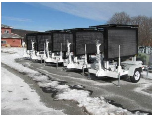
Photo 4: Variable message signs
