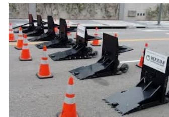
Picture 3: Modular vehicle barriers.
