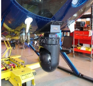
Picture 4: MX-10 camera system mounted to the underside of an HPD helicopter.
